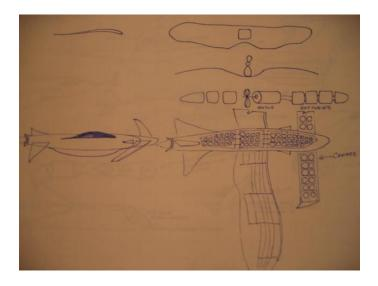
This concept above uses a polymer muscle with material memory coated with a solar powered film. Much of the design is based on nature, a bird, and takes into consideration the Anderson Number for the wing flapping sequence, note that the side view resembles a shark.
