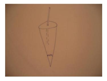
Can be used to drop communication devices into the ground from an air drop or to plant trees via UAVs.
