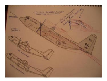
It has been theorized that the best aircraft to try this concept out on would be the C-130J Hercules and the C-160, although such a scheme could work on nearly any cargo aircraft with high performance turbo-props. Airflow over the wing would need a bit of assistance as well, perhaps using light-weight materials for large airflow guides.
